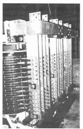
Internal connection failure on 18 MVA transformer.
