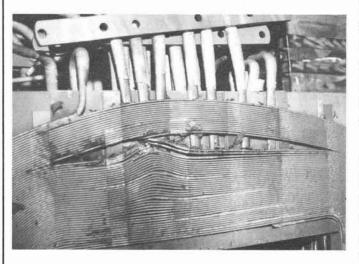
Shell type furnace transformer. High voltage winding, turnto-turn failure.
