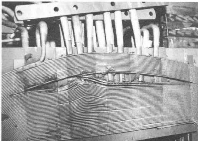
*Shell type furnace transformer. High voltage winding, turn-to-turn failure.*
