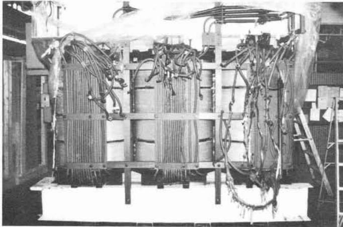
*Failure of extra flexible, high voltage connections.*
